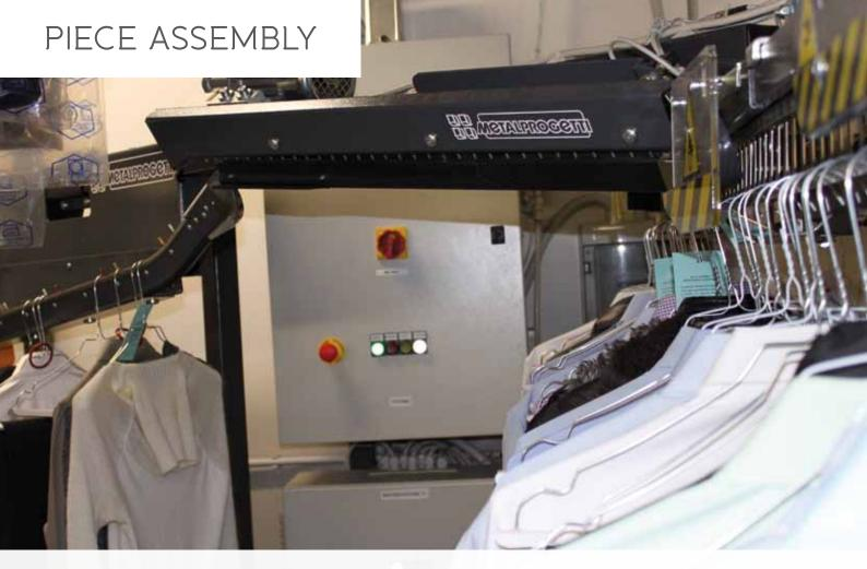
It automatically identifies and assembles one by one the garments of the order so that they are ready for delivery. It loads and unloads at the same time, avoiding downtimes. Very accurate, it increases productivity and reduces labour costs.
